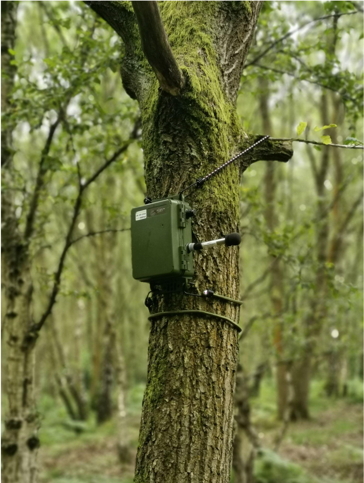
An autonomous sound recorder ready to monitor biodiversity in the UK. Copyright Carlos Abrahams.
